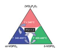
**Phased out**: The nature of the active layer in vanadyl pyrophosphate, a catalyst for *n*-butane oxidation to maleic anhydride, is a function of the atomic phosphorus/vanadium ratio in catalysts and of the temperature of reaction (see figure).
