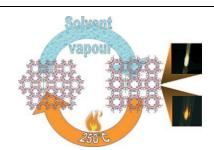
Switch your MOF: Metal-organic frameworks (MOF) of cluster [Cu<sub>4</sub>I<sub>4</sub>-(DABCO)<sub>2</sub>] have been prepared and characterized as two different crystalline forms, I and II. MOF I converts into II on exposure to acetonitrile or methanol vapour, whereas II reverts to I when heated in a closed pan at 250 °C (see figure). Both isomers exhibit luminescence properties in the solid state and these have been characterized at room temperature and at 77 K.
